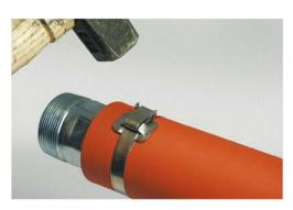
Hold stub of band with thumb, hammer it flat over bridge of buckle, complete clamp by hammering ears over stub.
