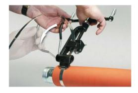
Pull on cutter lever, band is cut off to correct length.
