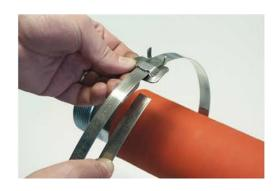
Pull buckle on band, ears pointing towards end of band. Form clamp, holding band on band, then push buckle back over the doubled band, bending the end approx. 1" under buckle.
