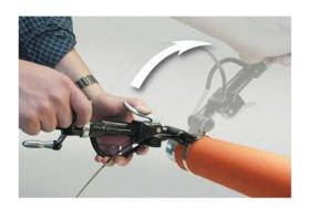
Place band in tool, push down on gripper with thumb, tension clamp by turning handle. Maximum tension is reached when band stops moving through buckle. When required tension has been applied, roll tool over buckle, at the same time reversing handle carefully approx. half turn to avoid breakage. There is no loss of tension, if handle is not reversed too much.
